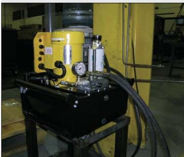
Z-class pump model number **ZW5020HK-FHT01** is used to provide pressure and flow to six machining fixtures.
