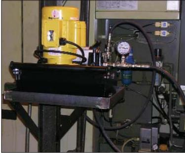
Z-class pump model number **ZW4210MB-FS** is used to provide pressure and flow to a single machining fixture.
